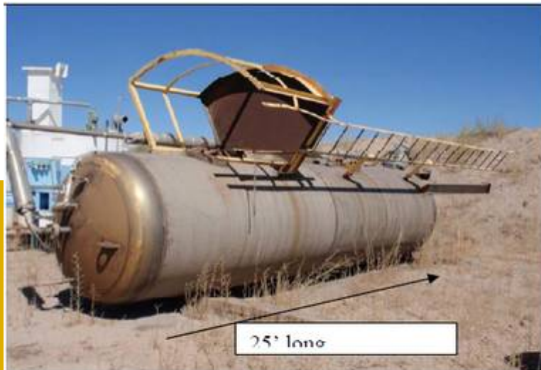
Precipitation Tank. 25' long, 5' diameter. The tank sets on 8"x8" posts
