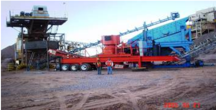
CONE CRUSHING UNIT OF 1500TONS FOR SHIFT IN LA HERRADURA
