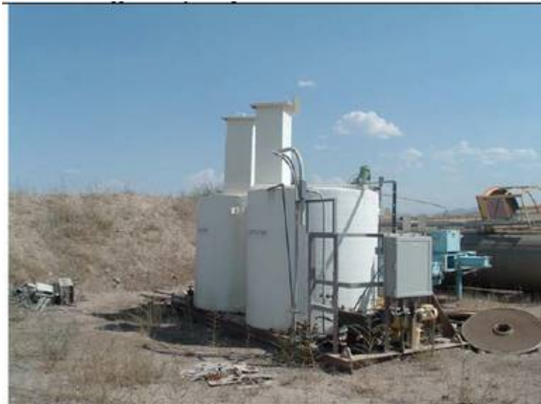
Water Filters – set on a skid. The skid is 22' long and 3' wide
